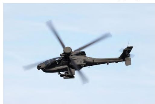
Apart from these changes, two major improvements over the old RNLAF AH-64DN are the FCR (Fire Control Radar) and the Link 16 capability. The Dutch air force will get ten FCR's and these will give the crew a much improved search capability. The FCR is housed in a radome on top of the main rotor. The Link 16 system will give the Apache the capability to share and receive real life information with other platforms during a mission.
